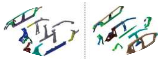
Fig.4Side wall explosion photos of split type (left) and integral type (right)
